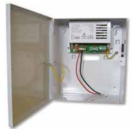
WBXPSU3A12VT (3 Amp) 13.8V Switch Mode PSU in Metal Box • Tamper Lid & Rear • Mains, Battery, Output & Fault LED • Enclosure - 200 x 240 x 75mm • Battery Compartment - 190 x 130 x 70mm
