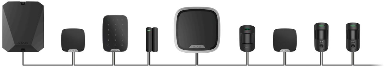
**Ring connection method** occupies two line outputs of the hub. If the ring breaks in one place, no device will be disabled. The ring reconfigures into two lines, which continue to operate normally. Users and security company will receive notification of a break.
