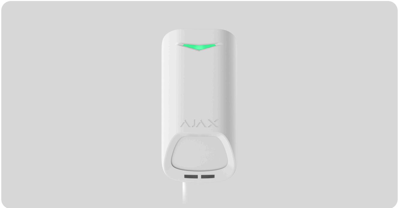
**Superior MotionProtect G3 Fibra** is a wired motion detector. It detects movement at a distance of up to 49 ft. In addition to using the IR sensor, the detector applies an additional radio frequency scan with a K-band microwave sensor that filters out infrared interference. Also, it features an anti-masking system that detects attempts to block the detector's field of view. The device is designed for indoor use only and complies with EN 50131 (Grade 3) requirements.
