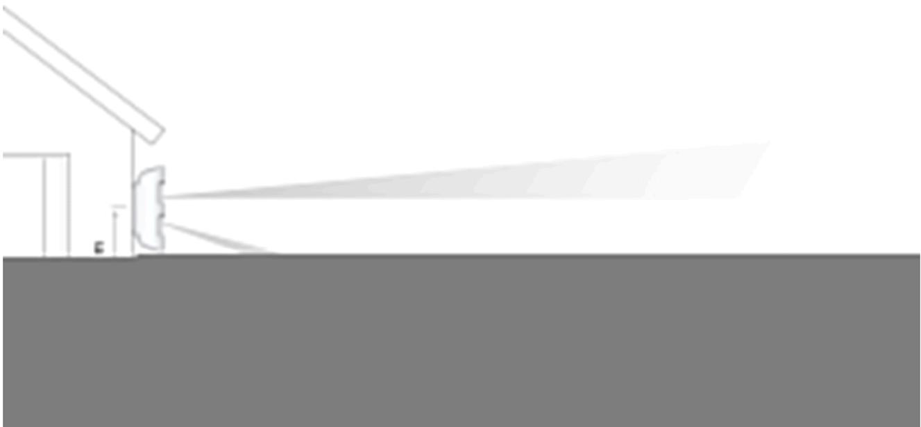
We recommend placing the detector in a corner so that it has no “blind” zones and is harder for an intruder to bypass. For example, in the corner of a fence. Furniture, plants, and ornamental and glass structures should not obstruct the view of the detector or its camera.
