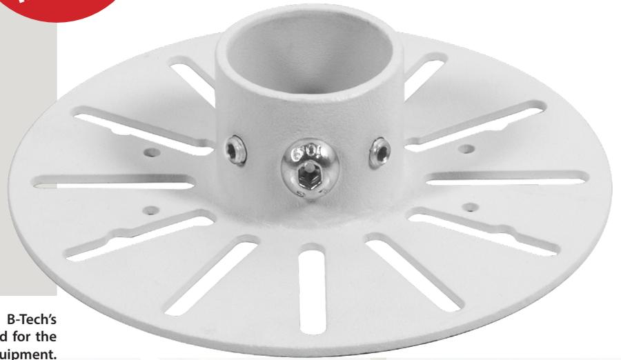
The BT5910 is a CCTV dome camera mount from B-Tech's System V Range; a collection of components designed for the installation of CCTV and other ceiling mounted equipment. Designed for use with BT5935 ø38mm poles, the mount can support a small to medium-sized dome camera up to 5kg and when used with other parts from the System V Range, allows professionals to customise their ceiling mounted security solutions to their specific requirement.
