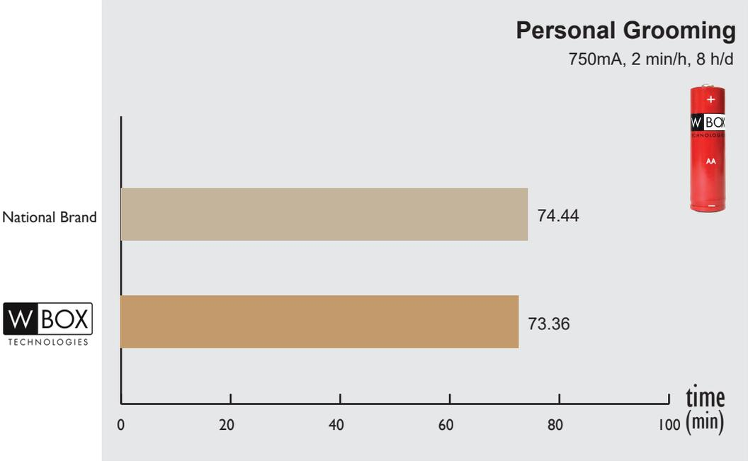
Remark: Battery discharging performance results from SGS report. Test conditions under ANSI Standard.
