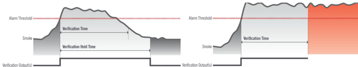
*Signal cleared before Verification Time expires – no signal. Without Verification Hold Time the panel would return to normal as soon as the signal dropped below alarm threshold.*
