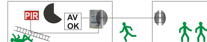
that is needed, no other ancillary devices are needed though a repeat AV indicator(s) with OK acknowledge buttons may be of benefit for the worker depending on the size of the working area. An alternative to an OK button would be one or more Passive Infra Red detectors, this could allow for hands free operation.
