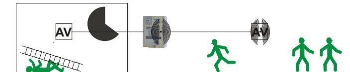
A MAYDAY and possibly an AV indicator within earshot of the responder are all that is needed, no other ancillary devices are needed though repeat AV indicator(s) may be of benefit to the worker. In this scenario the OK button on the front panel of the MAYDAY should be disabled (see below).
