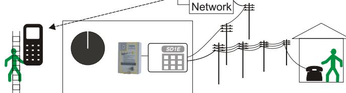
If an auto-dialler SD1E is used for communication as in scenario 3 then it is possible to use the communication link to enable the worker to use a mobile phone to generate an OK signal to restart the countdown timer. This would enable say a patrolling security guard to cover a large site without the need for dozens of hardwired OK/AV acknowledge buttons. Optional OK/AV buttons can be used if necessary to enable the countdown timer to be reset.
