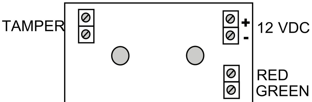
The PCB can be removed by gently levering it out along the top edge. The spares bag contains two wood screws & wall plugs to enable mounting. To refit PCB press it into the case gently bottom edge first.
