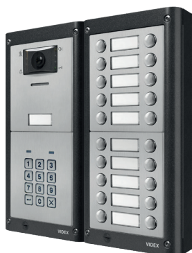
4 modules installation example with 1 video speaker unit, 1 codelock and 2 modules 4845D/M for 20 total push buttons
