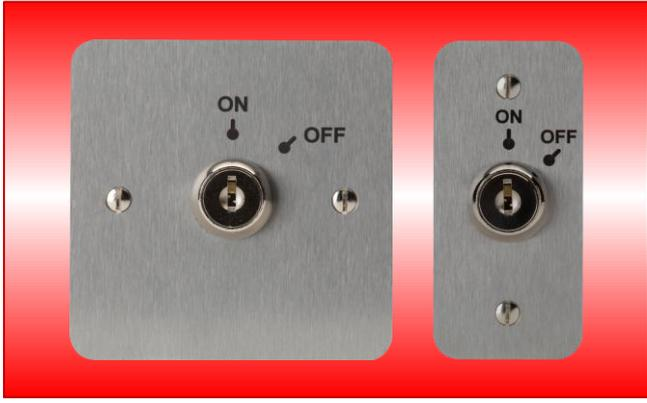
The 0660 keyswitch offers high reliability at an economical price. Momentary contact, spring return, providing 1 x normally open, 1 x normally closed circuit and 1 x common.
