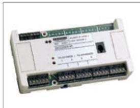
When a call is made from an outdoor panel, the MDS address corresponding to the house dialled is created, so that only the decoder with an output programmed with the MDS address generated will enable communication between panel and home.
