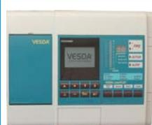
Central element of the ASD product range. VESDA VLP is classed as a “Very Early Warning Smoke Detector”, which means that it detects fire at the earliest possible stage and reliably measures very low to extremely high concentrations of smoke. Has an alarm sensitivity range of 0.005%–20% obs/m (0.0015%–6.25% obs/ft).
