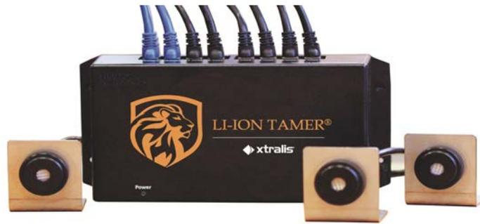
The Li-ion Tamer Rack Monitor system is a gas detection solution that enhances the safety of lithium ion batteries installations. It provides an alert to the venting of electrolyte solvent vapours (off-gas phase) that occurs early in the failure mode of li-ion batteries well in advance of smoke detection and traditional LFL gas detectors. The early detection of this event allows proper mitigation steps to be taken to avoid a catastrophic thermal runaway failure.
