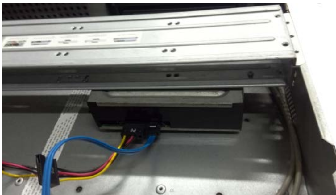
Figure 3-46 Connect cables
