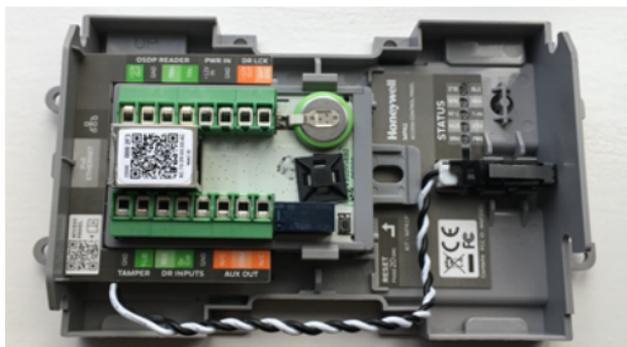
The inner base (with MPA1C1) can now be mounted on other devices or in a metal cabinet, using 2 or 4 short cabinet mounting screw supplied in the accessory bag.
