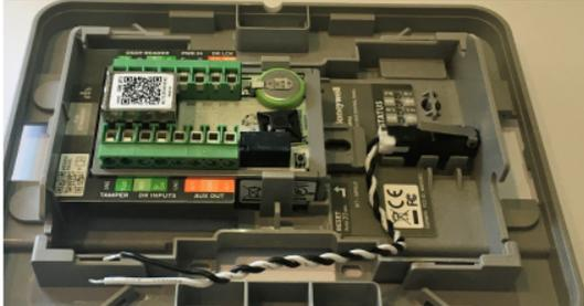
**Note:** The MPA1C1 Controller has been installed already in the MPA1ENCP enclosure.
