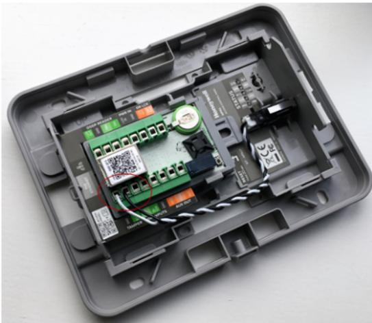
**Note:** *There is an additional internal accelerometer tamper switch that will detect any movement from the wall or from a gang box*
