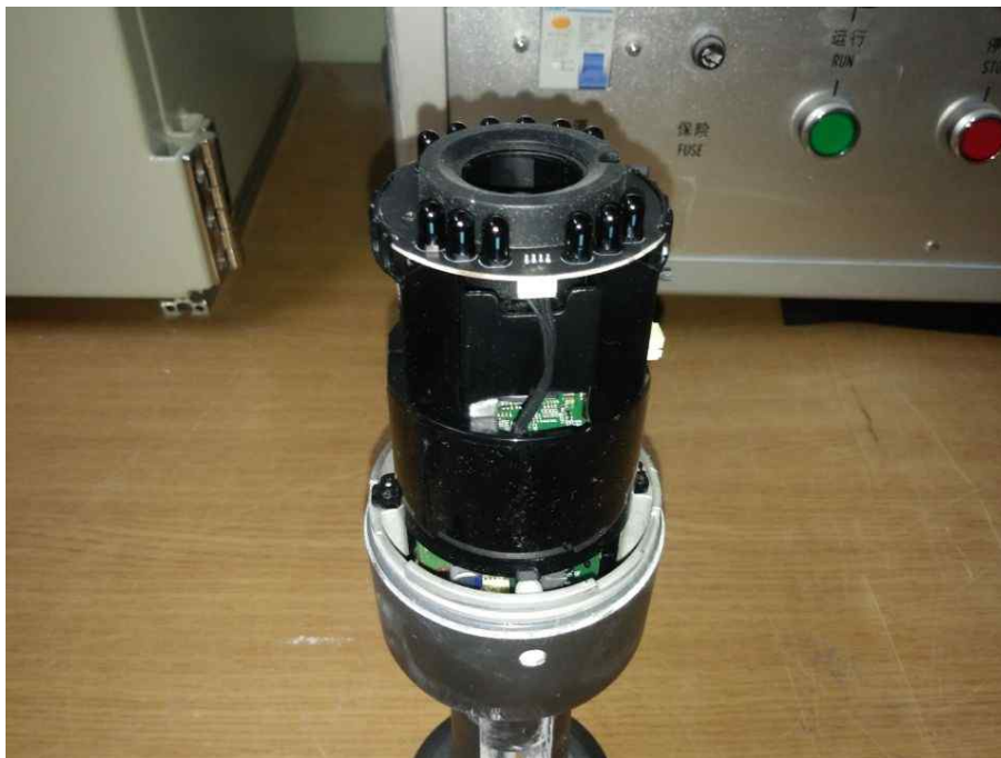
< Photo 9 > The second characteristic numeral test
