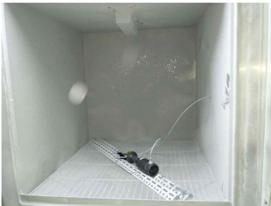
< Photo 6 > The second characteristic numeral test
