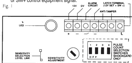
When using the sensor in momentary mode, it will usually be necessary to connect using a 6 core cable. If the latch facility is being used an additional core will be required for the connection of the latch terminal.
