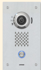
IX-DVF IP Video Door Station Fixed camera Stainless steel panel Vandal resistant Flush mount (back box included)
