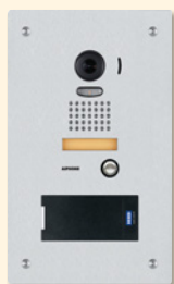
JP-DVF-RP10* Card Access Video Door Station • HID® multiCLASS SE® Proximity Card Reader • Stainless steel panel • Weather and vandal resistant • Flush mount (back box included)
