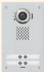
IX-DVF-4 IP Video Door Station Fixed camera Four call buttons Stainless steel panel Flush mount (back box included)
