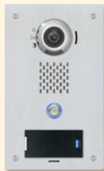
IX-DVF-P* Card Access IP Video Door Station HID® multiCLASS SE® Proximity Card Reader Fixed camera Stainless steel panel Weather and vandal resistant Flush mount (back box included)
