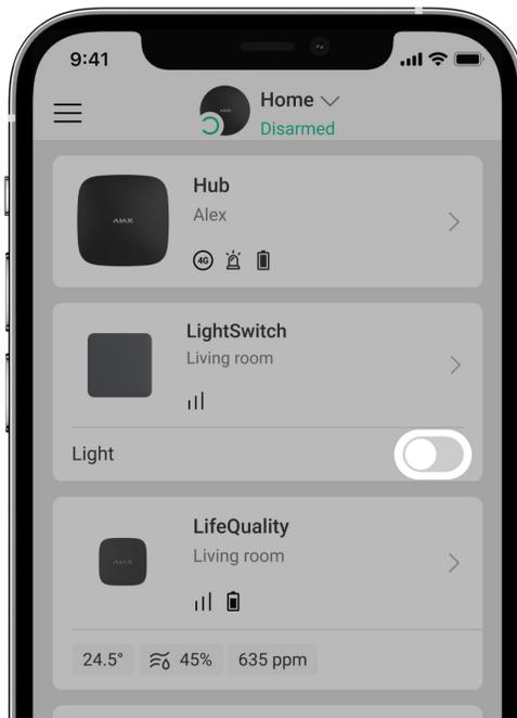
Press the switch in **LightSwitch** field in the **Devices**
