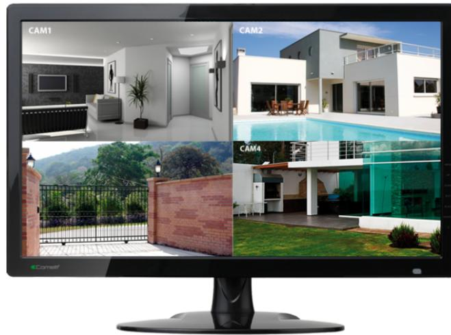
Colour monitor with 18.5" LED display, display ratio 16:9, HD resolution, 100/100 VESA mounting standard.
