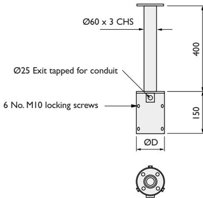
Commonly used for fixing cameras to the top of lighting poles
